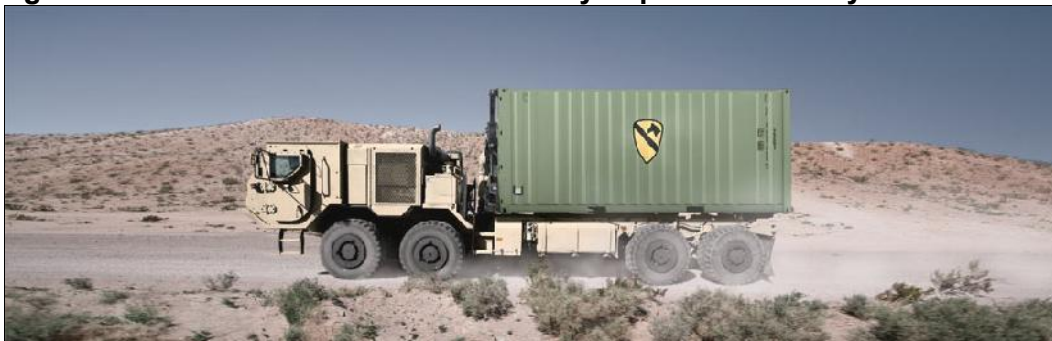
Figure 19: HEMTT A3 Diesel Electric Heavy Expanded Mobility Tactical Truck
